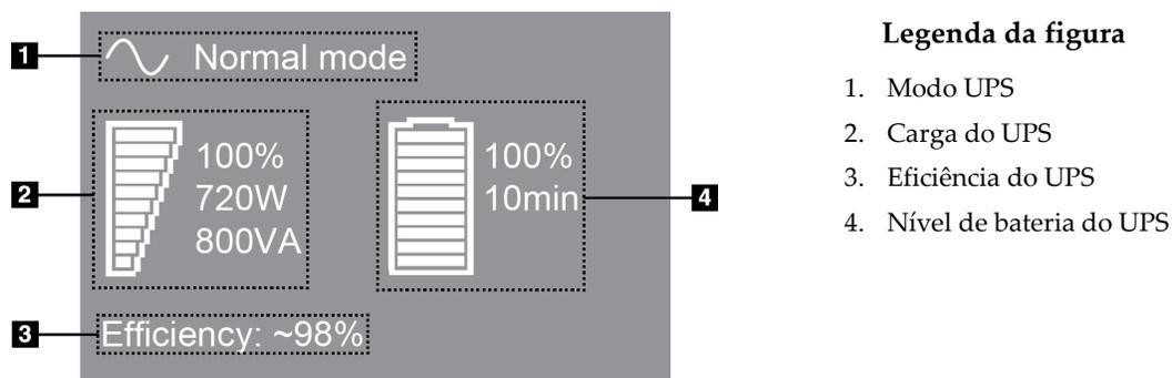
Figura 105: Monitor de LCD do UPS
