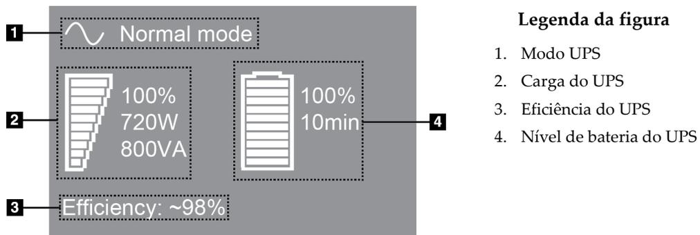
Figura 99: Monitor de LCD do UPS
