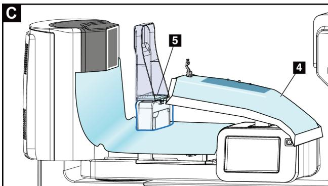
Install biopsy device mount drape section over biopsy device mount (item 4). Make sure the three protrusions and needle guide holder from the biopsy device mount line up with the respective openings in drape section. Peel off adhesive under drape flap (item 5) and attach to bottom of paddle.
