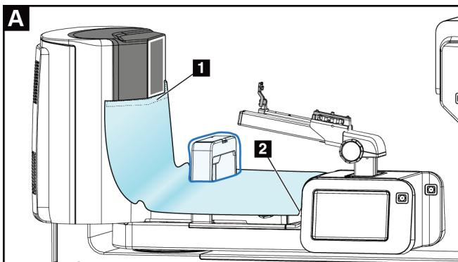
Install breast platform drape section on breast platform and over paddle mount. Peel off adhesive under drape (item 1) and attach to image receptor right below white square (do not cover white square area). Tear off excess drape at perforation (item 2) and save for later.
