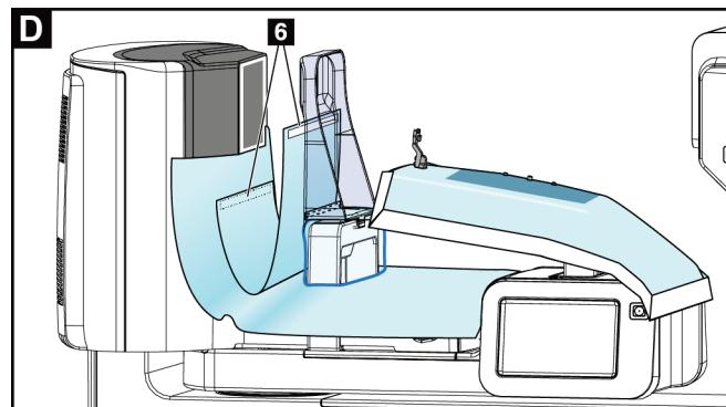
Locate previously torn off drape section and insert between paddle and breast platform to catch fluid leakage. Peel off adhesive on ends and attach to paddle and breast platform (item 6).
