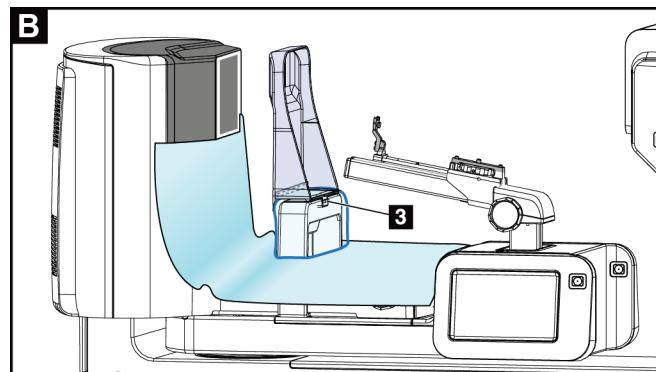
Attach paddle on the paddle mount (item 3) over the clear plastic pouch section of the drape.
