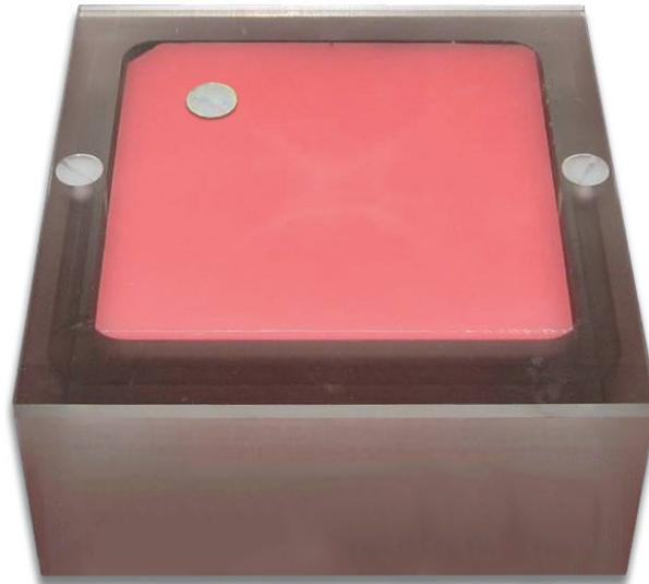
Figure 6: Placement of acrylic disc on phantom
