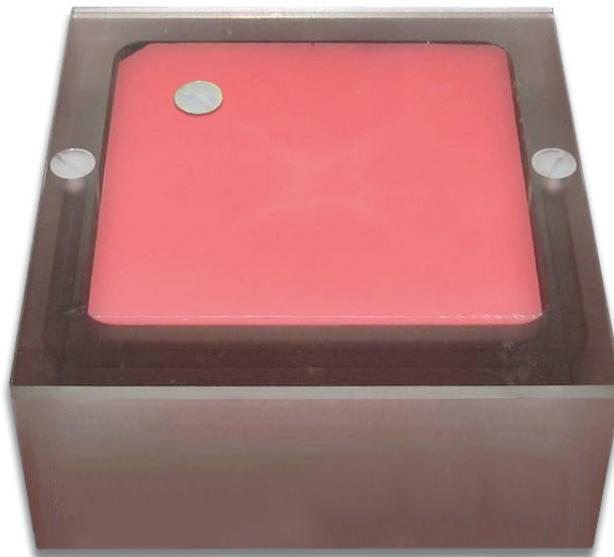
*Figure 7: Placement of acrylic disc on phantom*
