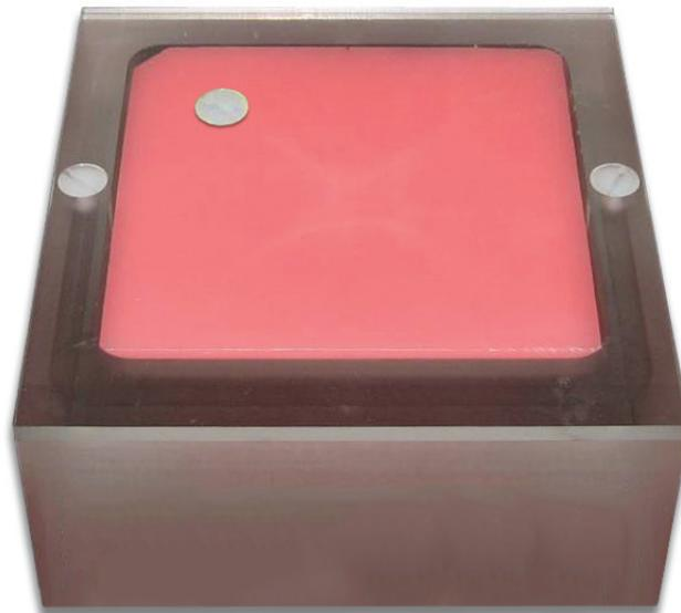
Figure 15: Placement of acrylic disc on phantom
