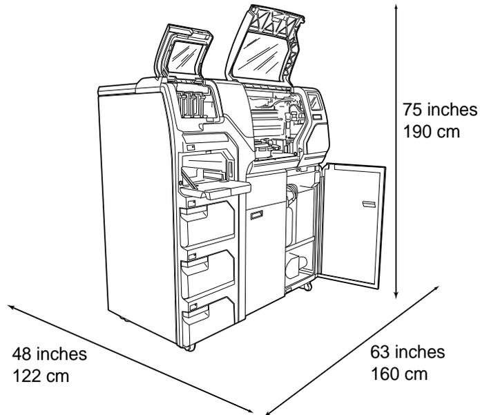
Figure 1-5 ThinPrep 5000 Processor with AutoLoader Dimensions and Clearances
