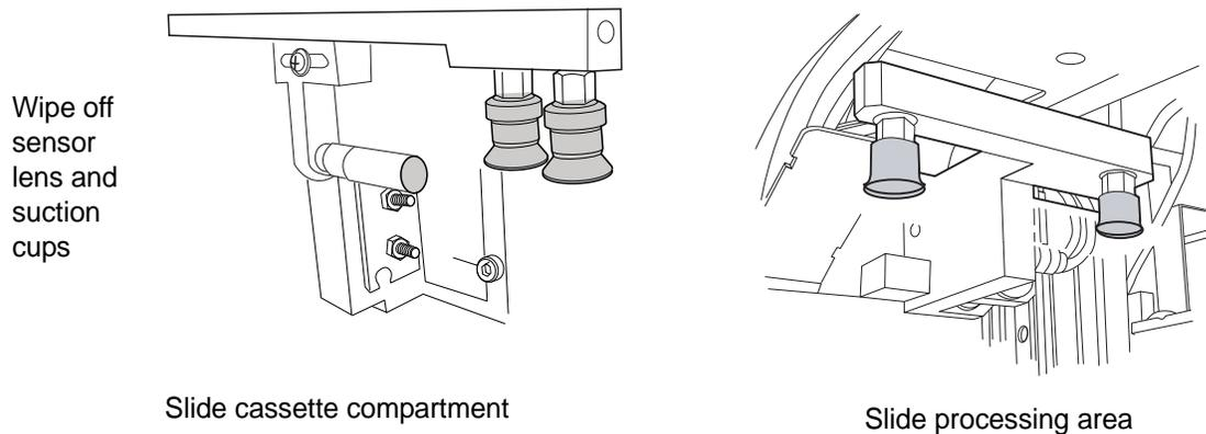
Figure 8-5 Clean Slide Holder Pneumatic Suction Cups
