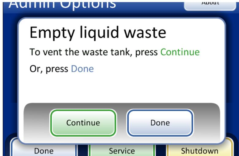
Figure 8-9 Empty Liquid Waste Button and Message
