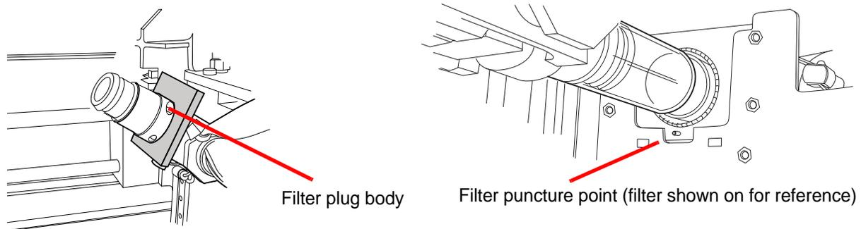
Figure 8-4 Clean Filter Plug and Filter Puncture Area
