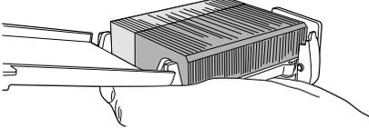
A line drawing showing a hand holding the cassette and looking at the slides inside to check their orientation.                                                   |
