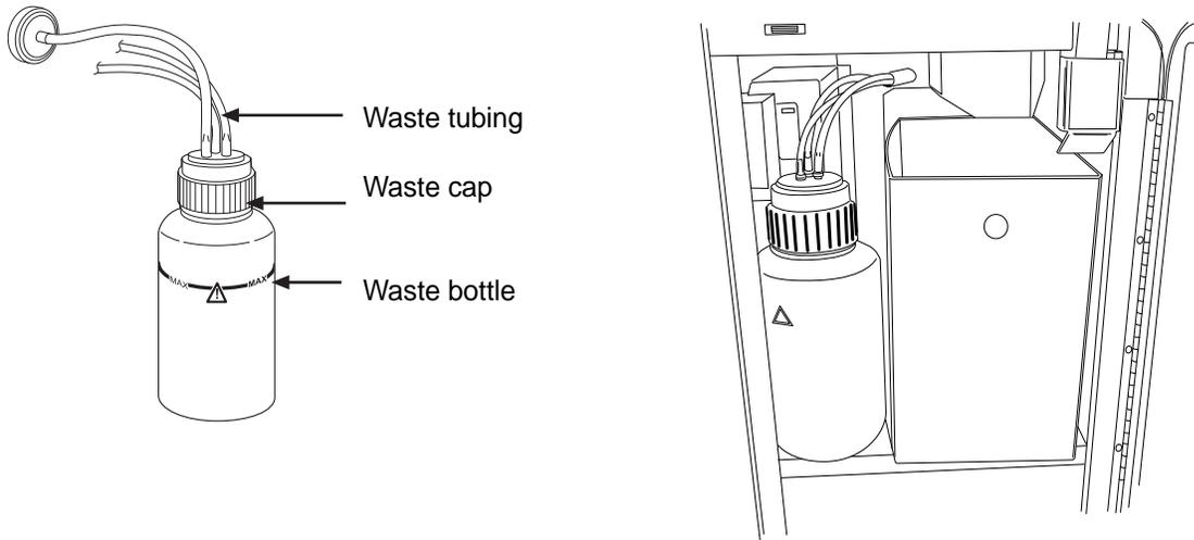
Figure 8-8 Waste Bottle and Waste Bottle Location
