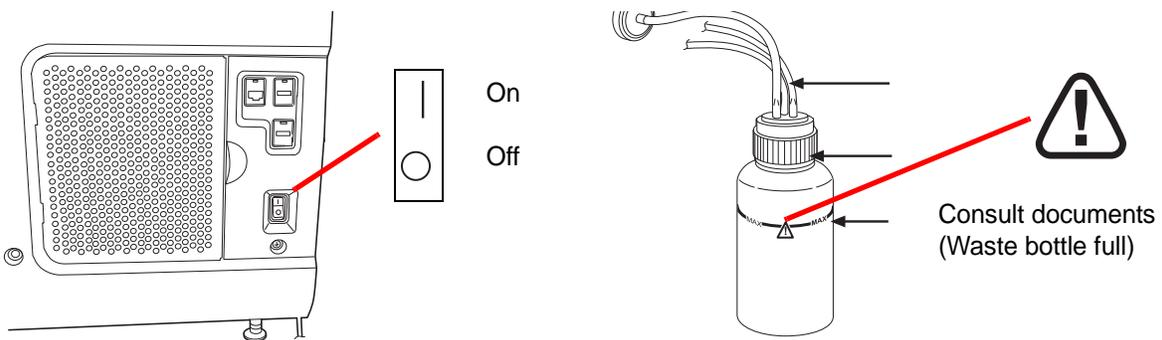
Figure 1-8 Right Side of Processor and Waste Bottle
