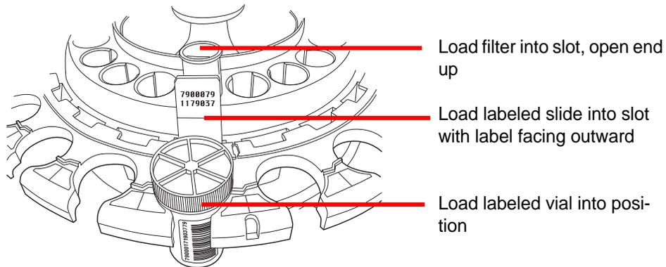
Figure 7-23 Load Carousel with Vials, Slides and Filters
