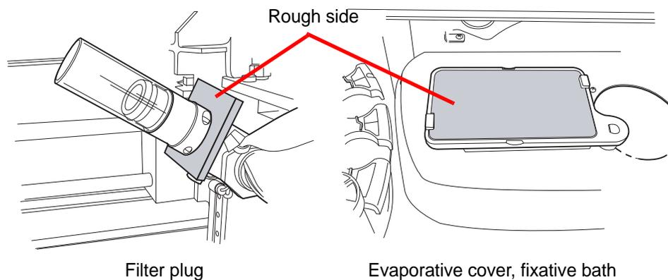
**Figure 8-17 Absorbent Pads**
