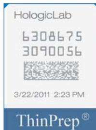
Figure 7-21 Example of a Laser Printed OCR Label on a ThinPrep Slide
