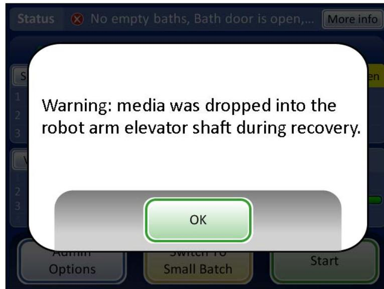
Figure 9-7 Media in the Elevator Shaft Message
