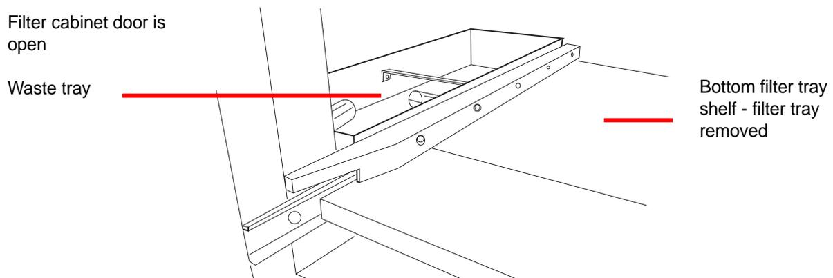
Figure 9-8 Robotic Arm Elevator Shaft Waste Tray
