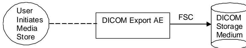
**Figure 5.1-1: Application Data Flow Diagram for Media Storage**
