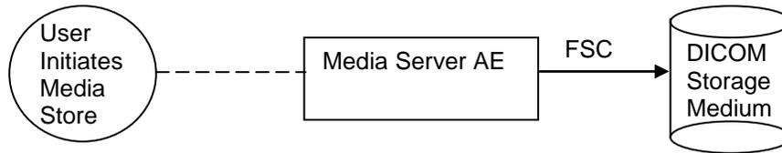
Figure 4.1-1 Application Data Flow Diagram for Media Storage
