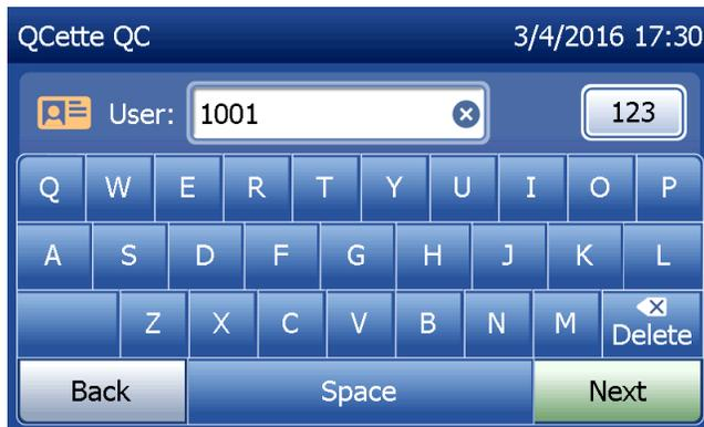
The QCette ID is displayed. (It was originally entered during QCette setup.) The QCette ID is the serial number for the QCette. Confirm that the serial number displayed matches the serial number printed on the QCette plastic housing and press **Next**. The software requires that the serial number is entered in the correct format: six numeric characters (e.g., 014899). Enter all leading zeros.
