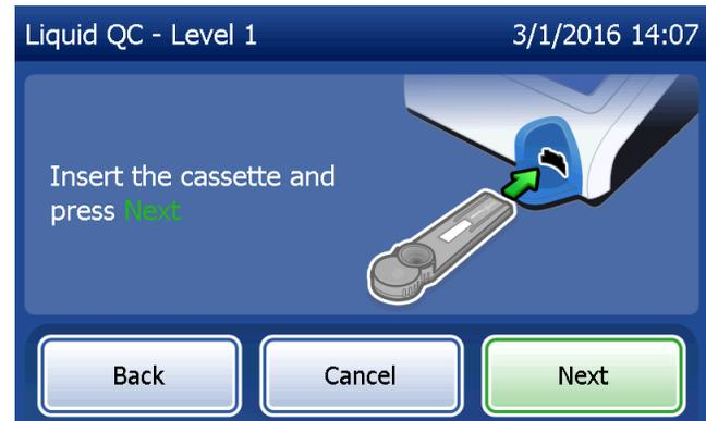
The analyzer will check that a Rapid fFN 10Q Cassette is properly inserted.
