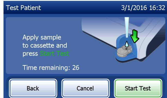
If the patient sample is not added and **Start Test** is not pressed within allotted time, the test process cannot continue. The display says that the sample was not added in time. Press **Close**, remove the cassette, and press **Finish** to return to the Main Menu. No record of the test will be held in memory.
