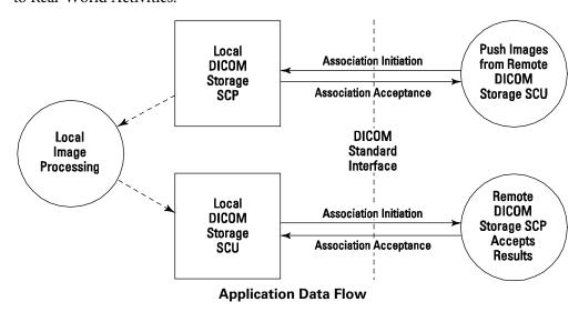
The Local Image Processing is initiated at system startup. The Local DICOM Storage SCU and local DICOM storage SCP are executed at system startup and exist in one executable program using two AE titles.
