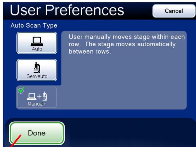
The user manually moves along the row using the stage control knob and pauses as desired. No speed settings are necessary.
