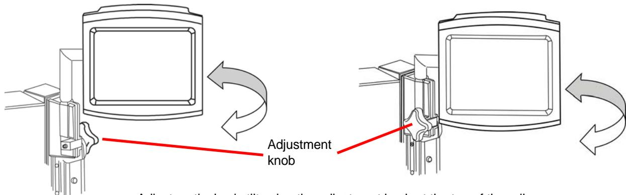
Adjust vertical axis tilt using the adjustment knob at the top of the rail.
