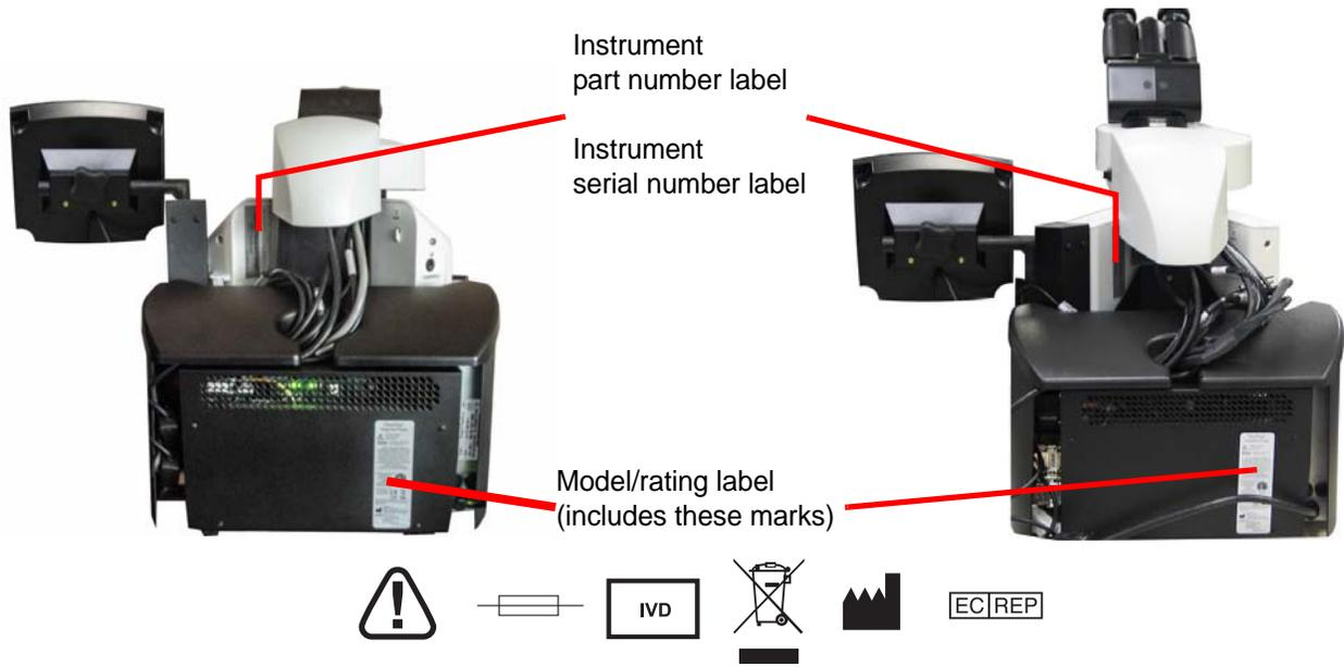
Rear of Instrument (PC removed for clarity.)
