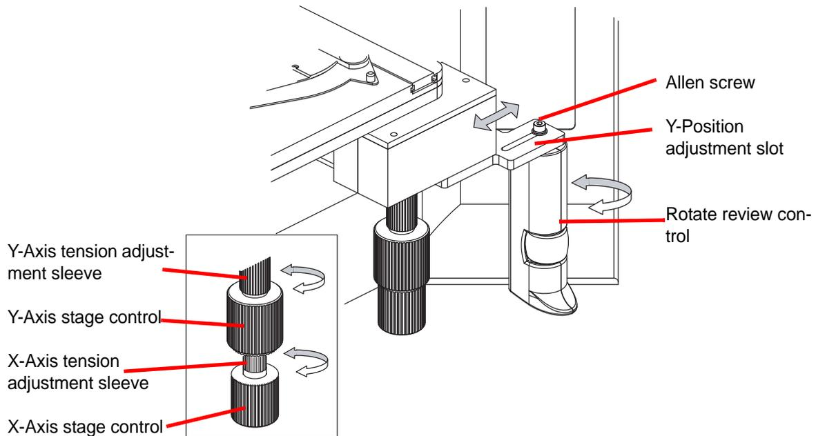
**Figure 2-5 Adjust Substage Controls**
