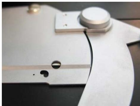
**Figure 5-1 Functional Check Features To Be Kept Clean**
