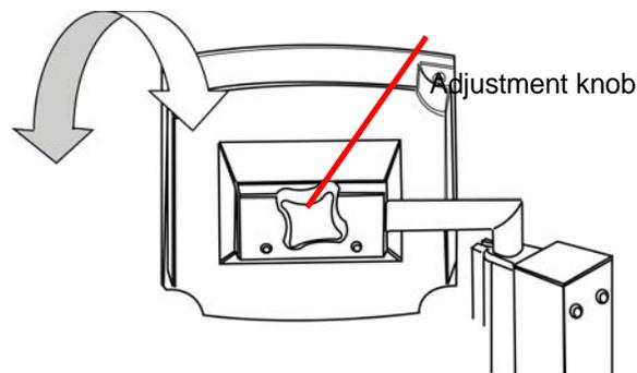
Adjust horizontal axis tilt using the adjustment knob on the rear of the screen.
