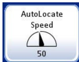
The Auto Locate Speed setting adjusts how quickly the stage moves from field to field during presentation of the 22 fields of view. The stage moves to each field of view and stops until the user presses the **Next** function.
