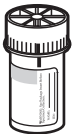
Line on cap and line on vial should meet or slightly overlap.
