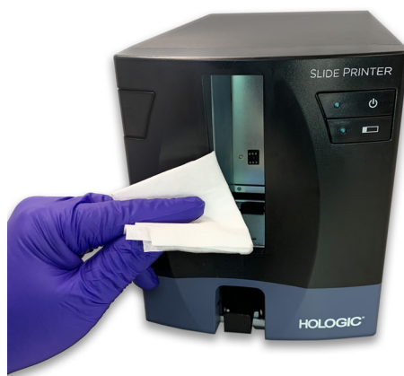
Figure 8-11 Clean the input roller on the slide printer
