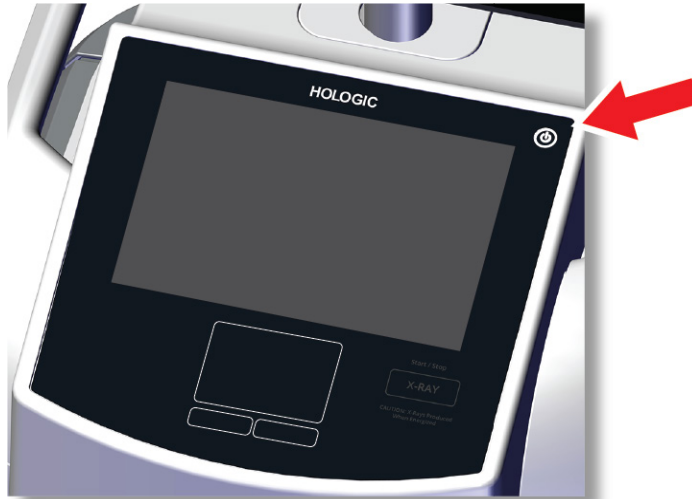
Figure 8: Computer Power Switch
