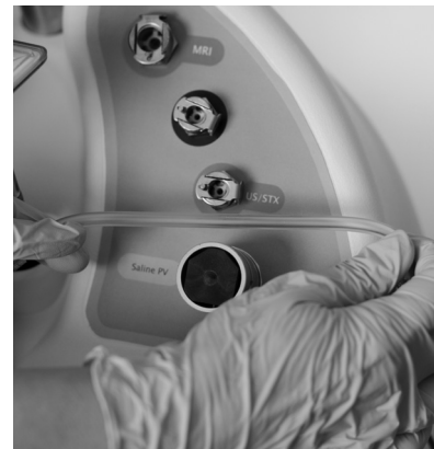
FIGURE 5: SALINE PINCH VALVE CONNECTION
