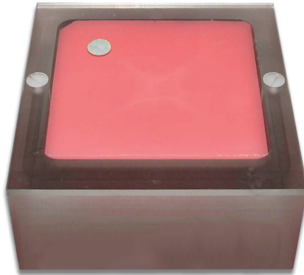
Figure 6: Placement of acrylic disc on phantom
