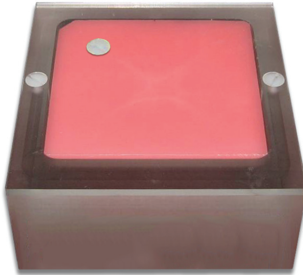
Figure 14: Placement of acrylic disc on phantom
