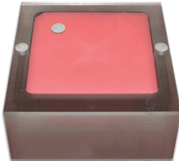
Figure 15: Placement of acrylic disc on phantom
