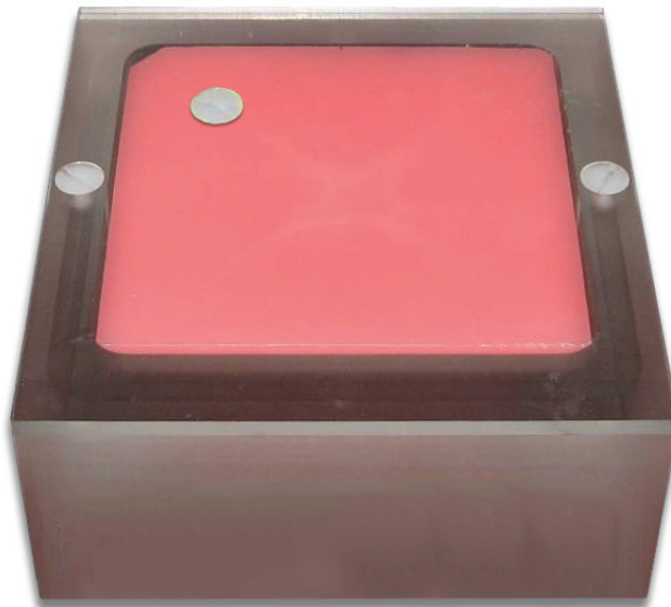
Figure 7: Placement of acrylic disc on phantom
