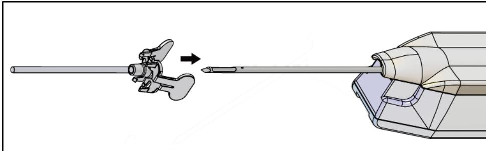
Figure 49: Slide the Introducer onto the Biopsy Device
