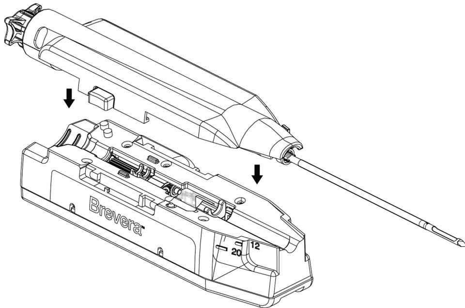
Figure 15: Biopsy Needle and Device Driver Connection
