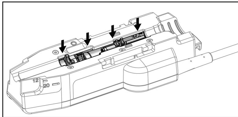
Figure 8: Metal Parts of the Device Driver
