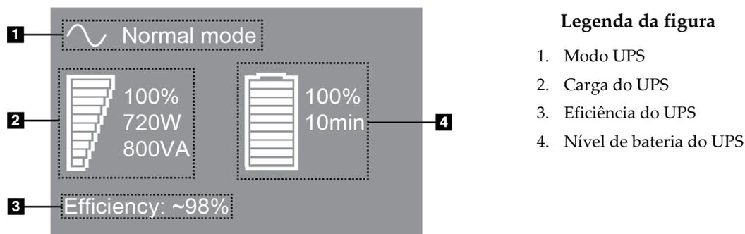
Figura 110: Monitor de LCD do UPS
