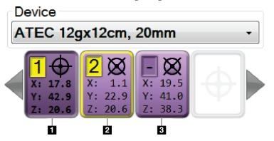
• The targets are now numbered and the target that is currently selected on the Acquisition Workstation [item 1 in preceding image] is shown depressed and the corresponding numbered target mark on the display monitor shown in the vertical (not tilted) position [see also item 1 in following image].
