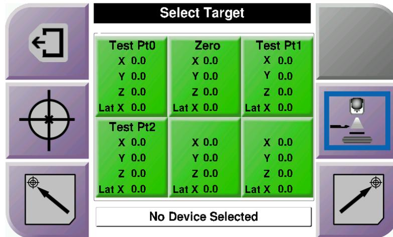
Figure 43: Select Target Screen for Lateral Arm
