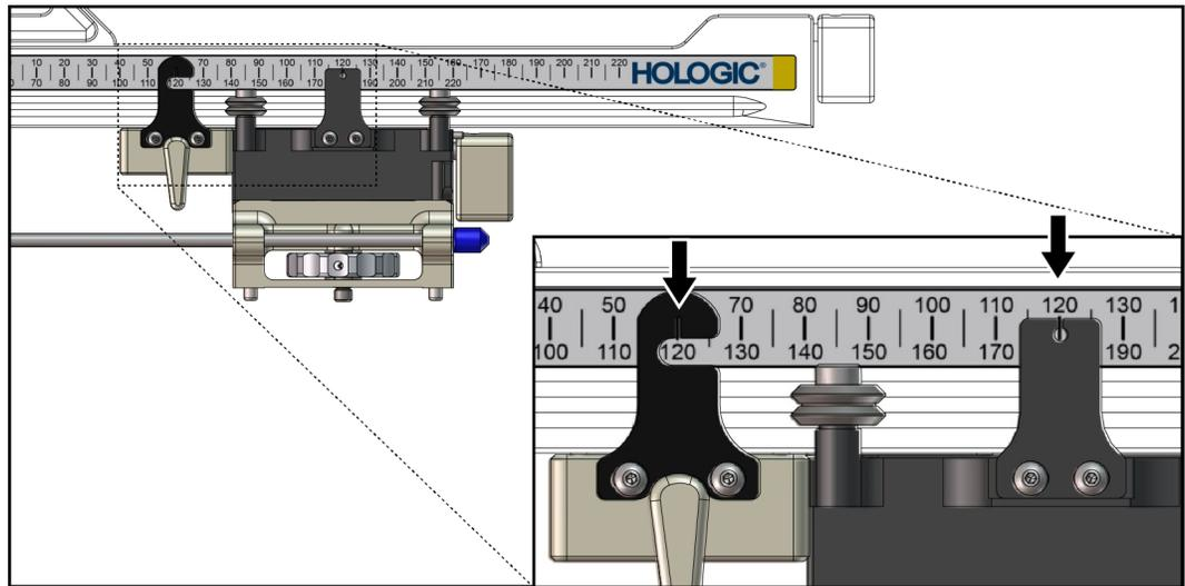
*Figure 28: Scales and Positioning for X-Stop and Carriage*
