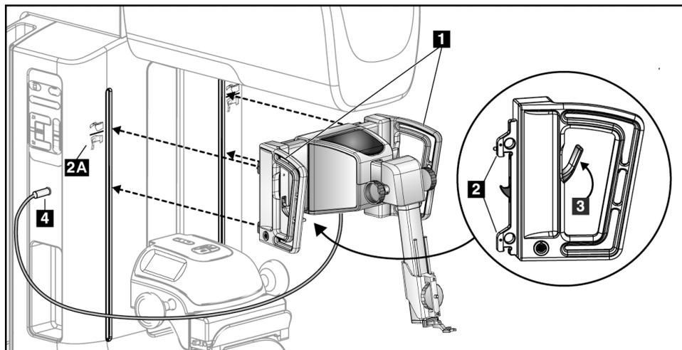
Figure 8: Installation of the Biopsy Guidance Module
