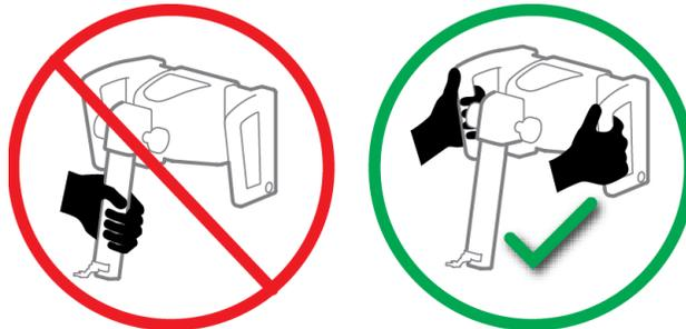
*Figure 2: How to Lift the Biopsy Guidance Module*
