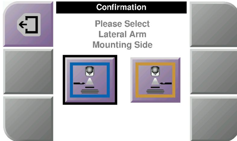
*Figure 19: Lateral Arm Mounting Side Selection Screen*
