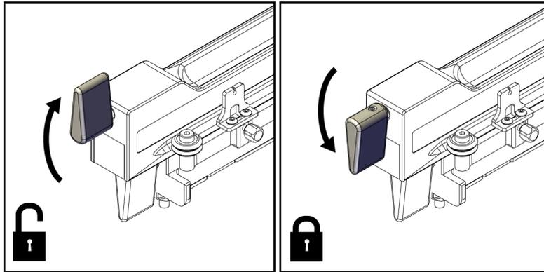
Figure 23: Carriage Lever Locked and Unlocked Positions
