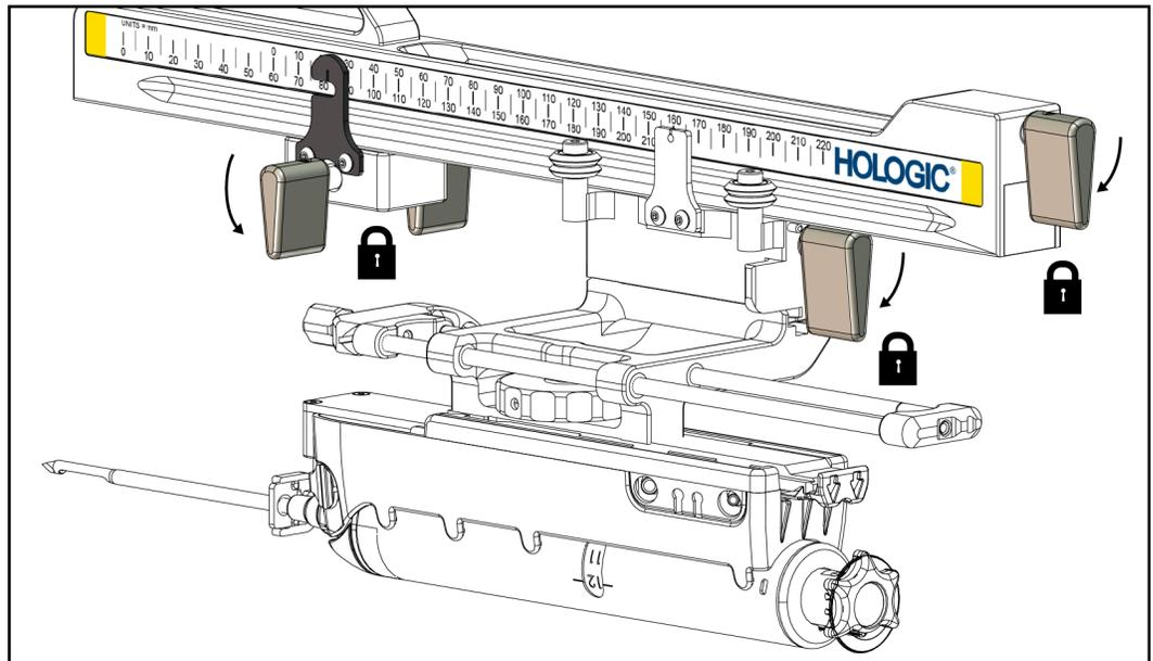
Figure 27: Lock Levers in Fully Locked Position
