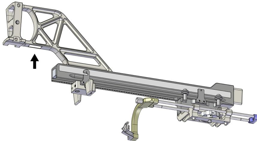
Figure 5: Lateral Arm Serial Number Label Location
