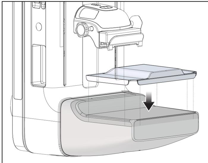
Figure 16: Installing Lateral Arm Stand over Image Receptor
