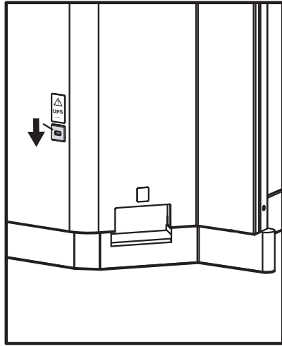
Figure 3-6: The Acquisition Workstation UPS Switch Lever
