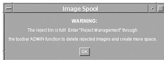
Figure 110: Reject Spool Full Alarm
