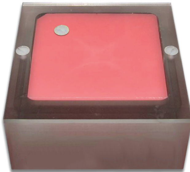
Figure 7: Placement of acrylic disc on phantom
