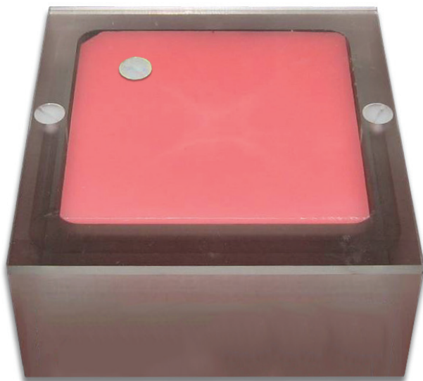
Figure 6: Placement of acrylic disc on phantom
