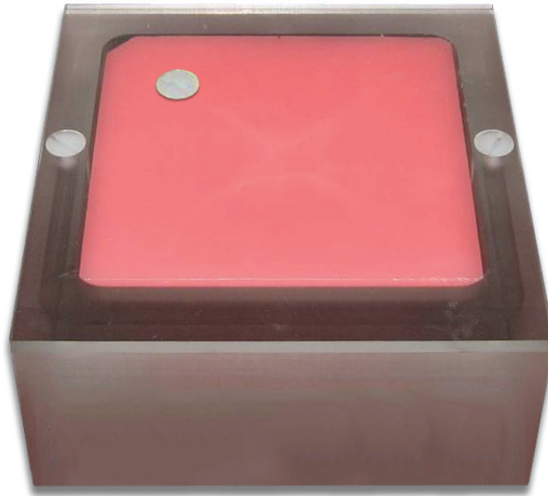
Figure 14: Placement of acrylic disc on phantom
