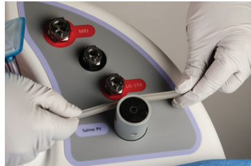
Insert clear section of saline tubing into Saline PV (pinch valve).
