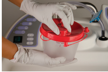
Make sure the canister lid is tightly sealed and the large cap is snapped onto the proper opening.
