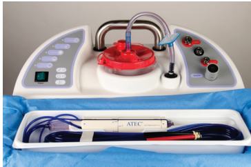
Place the handpiece tray into the top of the console and unfold the blue wrap.
