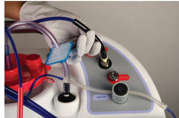
Connect the black handpiece line to the black handpiece receptacle located on the user interface.
