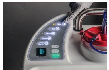
Choose "SET UP" and the "VACUUM READY" light will illuminate solid green when adequate vacuum is achieved. (At this time, verify the presence of saline in the tissue filter and needle aperture.)
