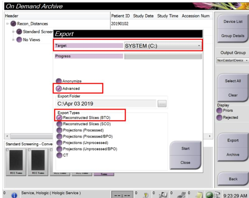
**Figure 3: Selecting Drive Location and Format Type for Images.**
