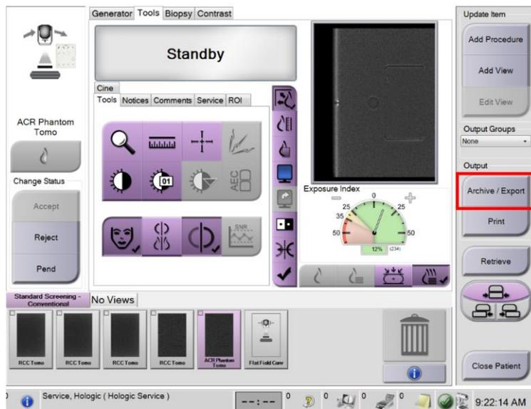
**Figure 1 - Exporting ACR DM Phantom Images in Procedure Screen**
