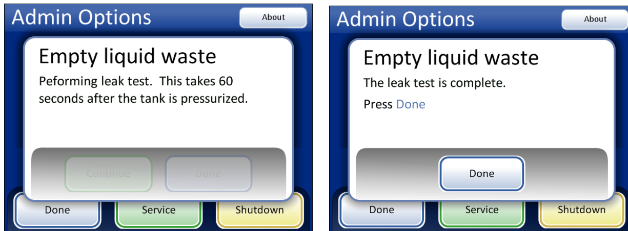
Figure 8-15 Waste System Leak Test
