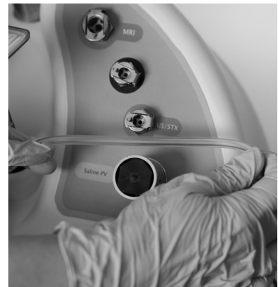
FIGURE 5: SALINE PINCH VALVE CONNECTION
