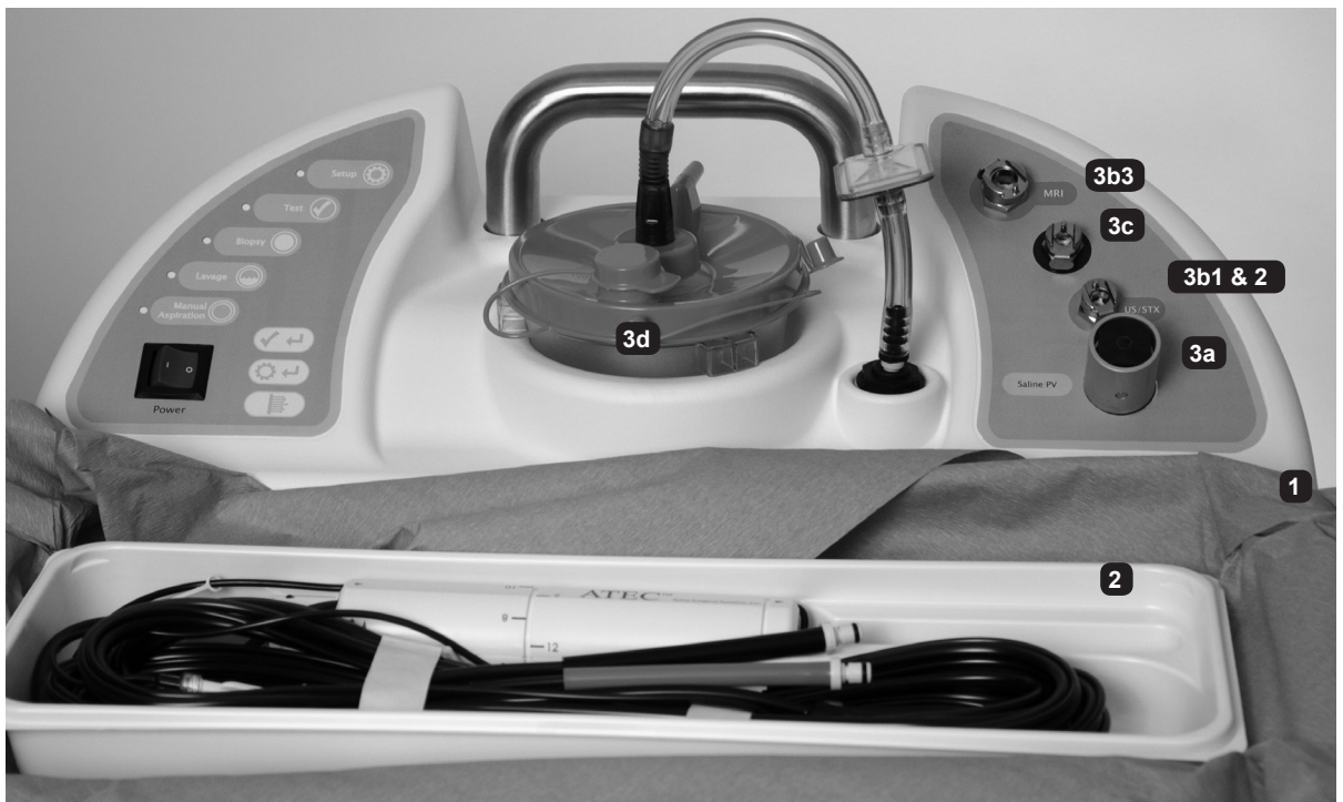
FIGURE 3: VACUUM AND HANDPIECE ASSEMBLY AND CONNECTIONS
