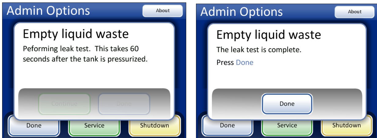
Figure 8-14 Waste System Leak Test
