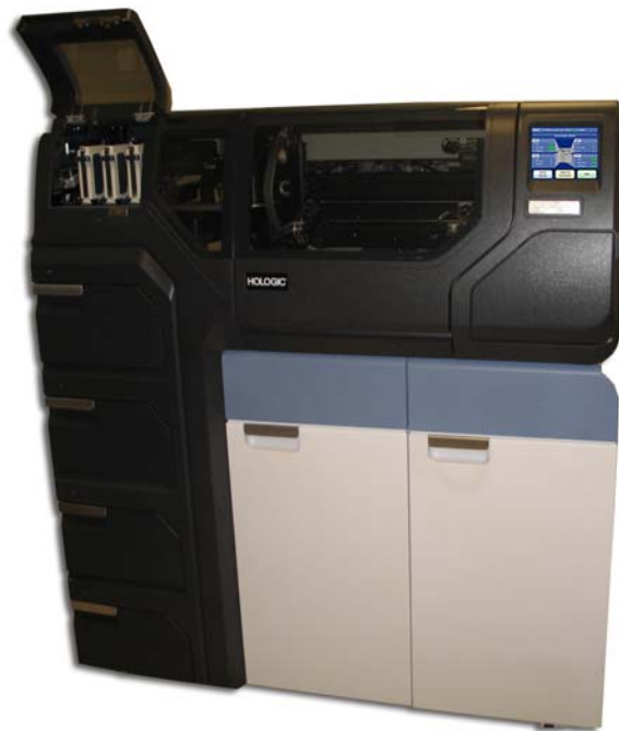
Figure 2-1 A Typical ThinPrep 5000 Processor with AutoLoader
