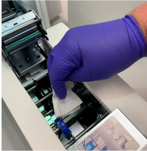
Figure 8-10 Wipe the slide printer transportation rollers
