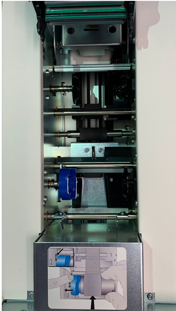
Figure 8-9 Slide printer transportation rollers
