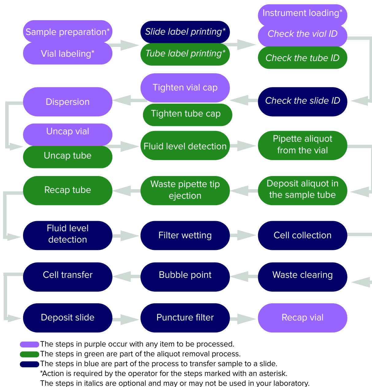
Figure 1-3 Slide processing and aliquot removal on the ThinPrep™ Genesis™ processor
