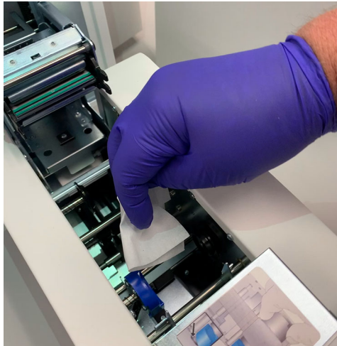
Figure 8-10 Wipe the slide printer transportation rollers
