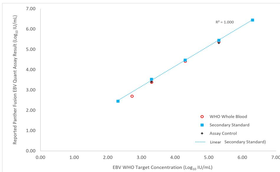
**Figure 6. Traceability Between the EBV 1st WHO Standard Target Concentrations and Reported Concentrations in the Panther Fusion EBV Quant Assay (WHO Standard Diluted in Whole Blood)**
