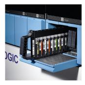
Random access enables loading samples with any test, any time eliminating batch constraints and decreasing turnaround time.
