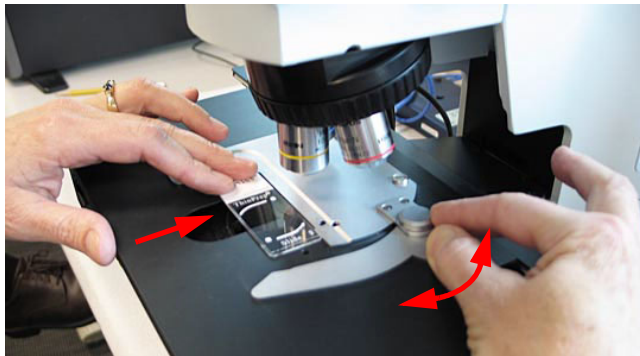
Use the button to open the slide clip. Load slide. Release the slide clip.
