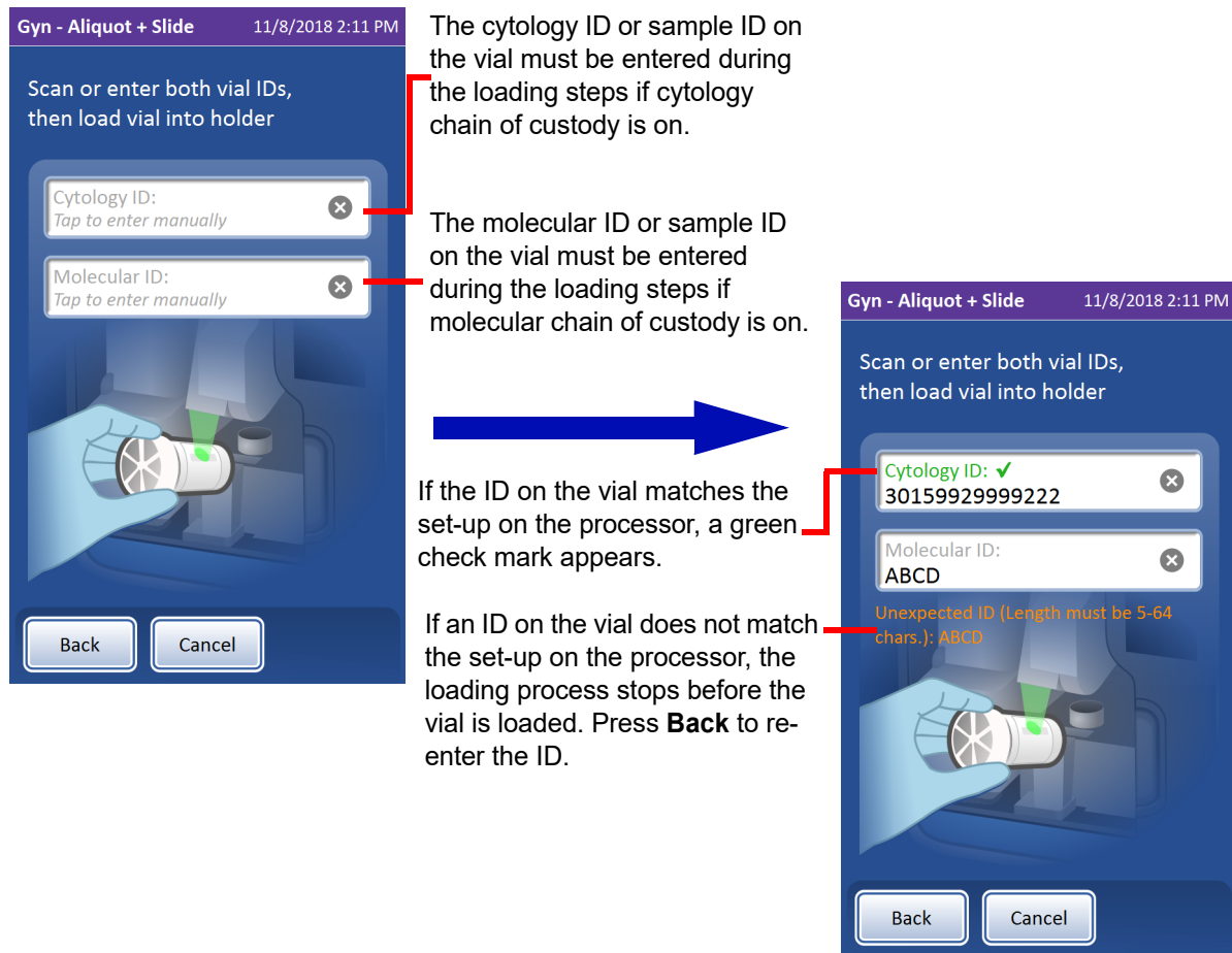
Figure 6-31 Chain of custody on - begin loading by entering ID(s) from vial
