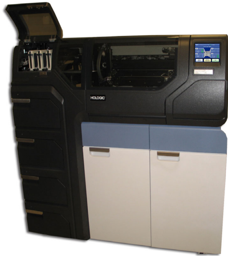
Figure 1-1 A ThinPrep 5000 Processor with AutoLoader
