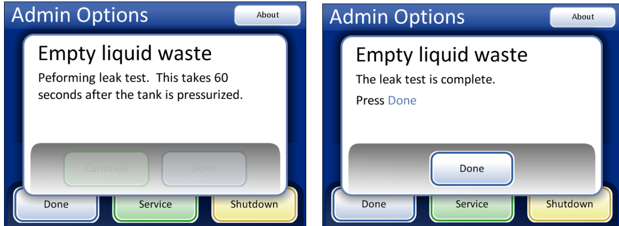
Figure 8-15 Waste System Leak Test
