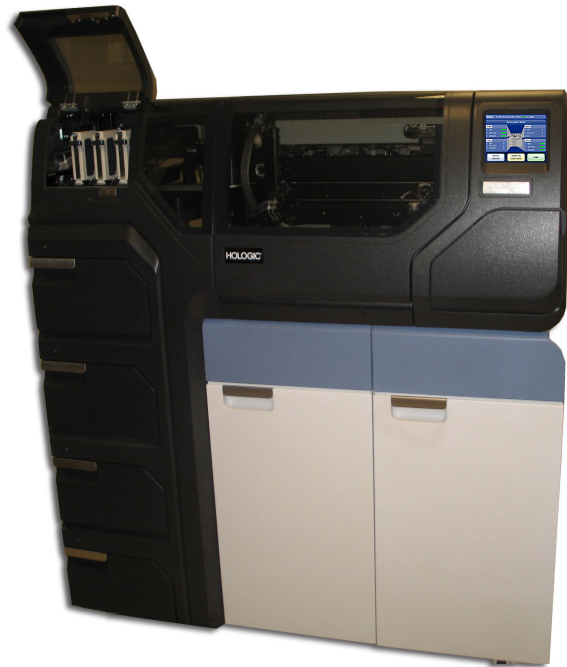
Figure 2-1 A Typical ThinPrep 5000 Processor with AutoLoader
