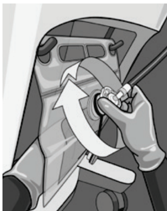
Figure 56: Install Waste Bag Connector
