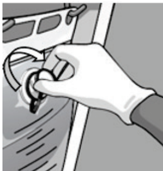
Figure 54: Screw Waste Bag Cap onto Waste Bag
