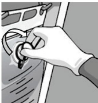
Figure 60: Screw Waste Bag Cap onto Waste Bag
