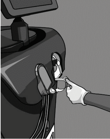
Figure 26a: Depress Out-FloPak Lever
