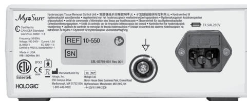
FIGURE 2. MYOSURE CONTROL UNIT—REAR PANEL (*=EQUIPOTENTIAL COMPENSATOR TERMINAL)
